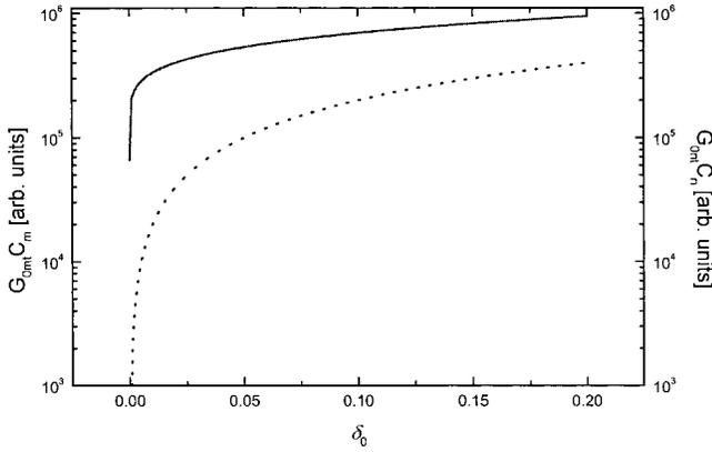
FIG. 2. Comparison of the threshold gain with and without mirror. Dashed line is for the system with mirror, whereas the solid line is for the system without mirror.  $C_m$  and  $C_n$  are two constants, which have comparable values.  $\delta_0$  stands for  $\delta_{0m}$  and  $\delta_{0n}$  for systems with and without mirror. It can be seen that the decrease of threshold would be weakened when  $\delta_0$  increase, but is still a large amount.
